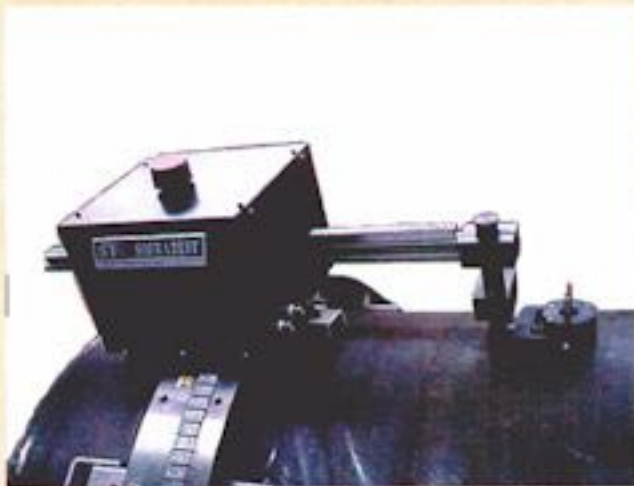
Sofrascan uses flexible track, here mounted on 700mm OD pipe -
