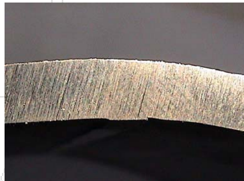
Example of weld after scarfing process
